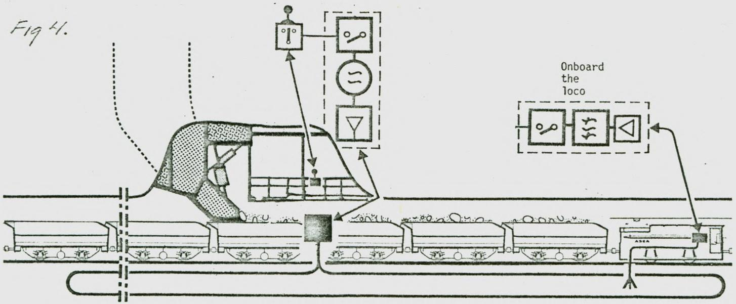
The basic requirements on the locomotive are that its brakes must be applied by means of electrical circuits and that the "Forward" and "Reverse" switching have to be electrically controlled as well as the selection of speed. For safe operation the brake system should be of "inverted" type, i.e. the brakes shall be applied at loss of power or loss of transmission from the transmitter. Modern type of thyristor controlled locomotives usually fulfil those requirements.
