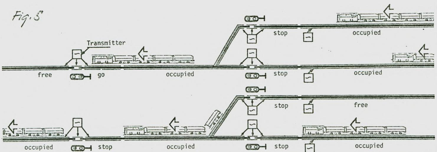
Each block is normally controlling two antenna loops. One loop ahead of the block limit and one after the limit. The former one transmits the state of the following block, the latter one the recommended speed within the block. If this block is occupied the former antenna is sending stop command. If the driver in such a case does not obey the red block approach signal, the emergency brakes on the loco will automatically be applied.
