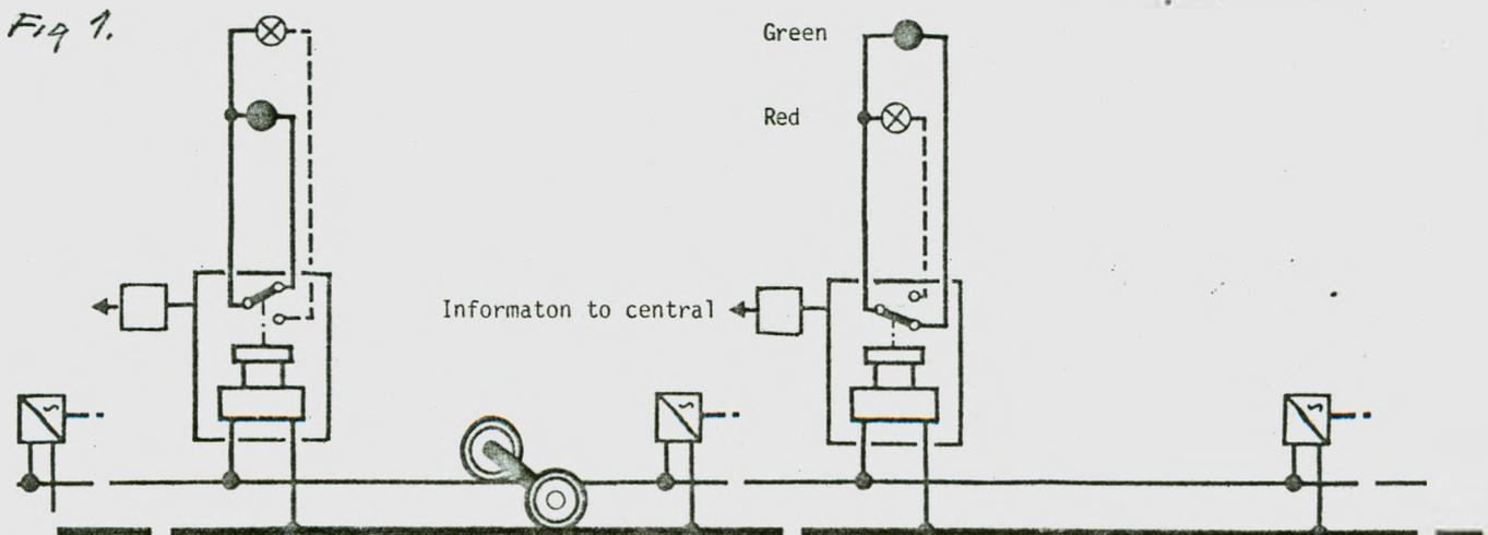
The function of this system depends on the condition of the track ballast. The system is working in mines with extremely good non-conductive ballast but cannot generally be used in wet mines. The system also requires good conductive connection between the wheels on the axles as well as "clean" rails, i.e. free from rust or other oxides.
