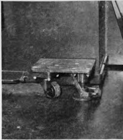
Caster and toe jack on C.T.C. machine
