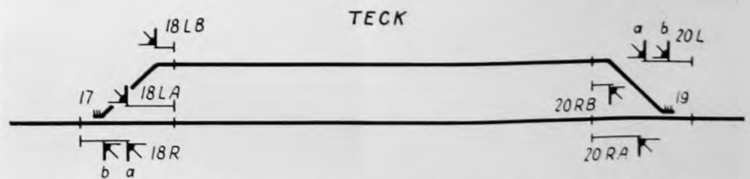
Fig. 2—Track and signal plan of the siding at Teck showing use of signals to save train time
