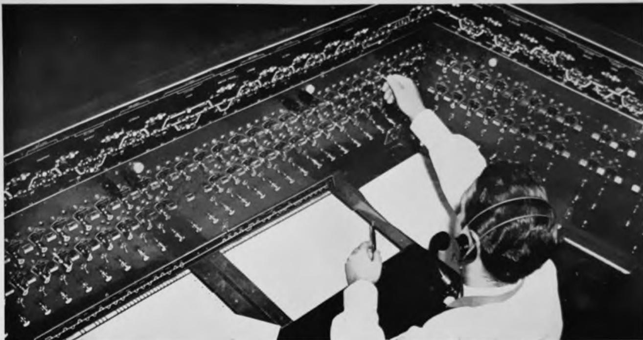
This C.T.C. machine in the office at Las Vegas, Nev., controls the territory between Caliente and Las Vegas
