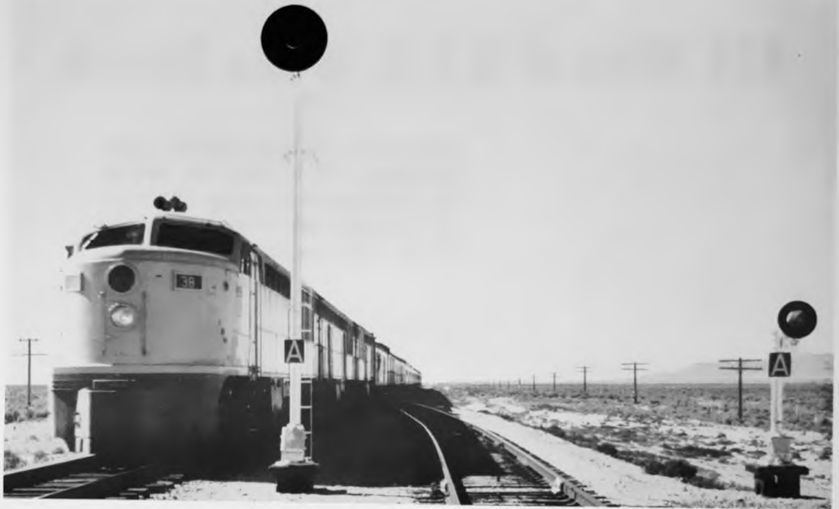
Above—View at a typical siding, including a power switch machine and C.T.C. controlled searchlight signals—of special interest is the “high” mast for the leave-siding dwarf signal
