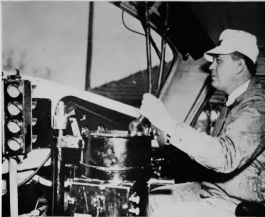
The cab signal in each Diesel-electric locomotive displays aspects faced to the engineman, and also to the fireman's side of the cab
