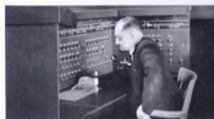
DISPATCHER connects "OS" marks on the train graph to make continuous record.
