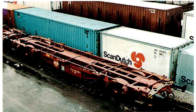
Two-axle special type wagon (class Lgjs). The frame is equipped with a long-stroke shock-absorbing device (length of stroke max 760 mm), which protects the container and the load in the case of shunting impacts.
