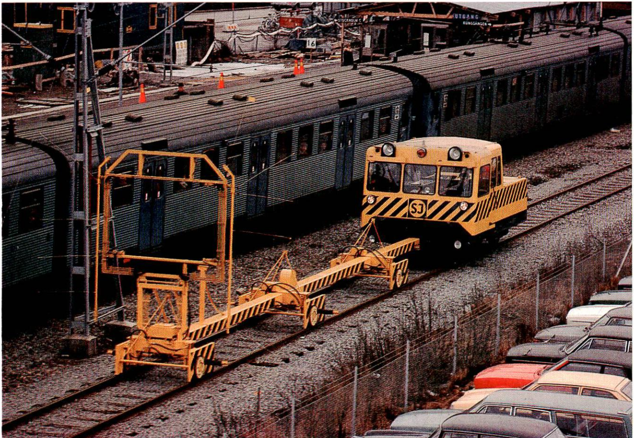
The STEFO recording car with its measuring trolleys with the reference points
