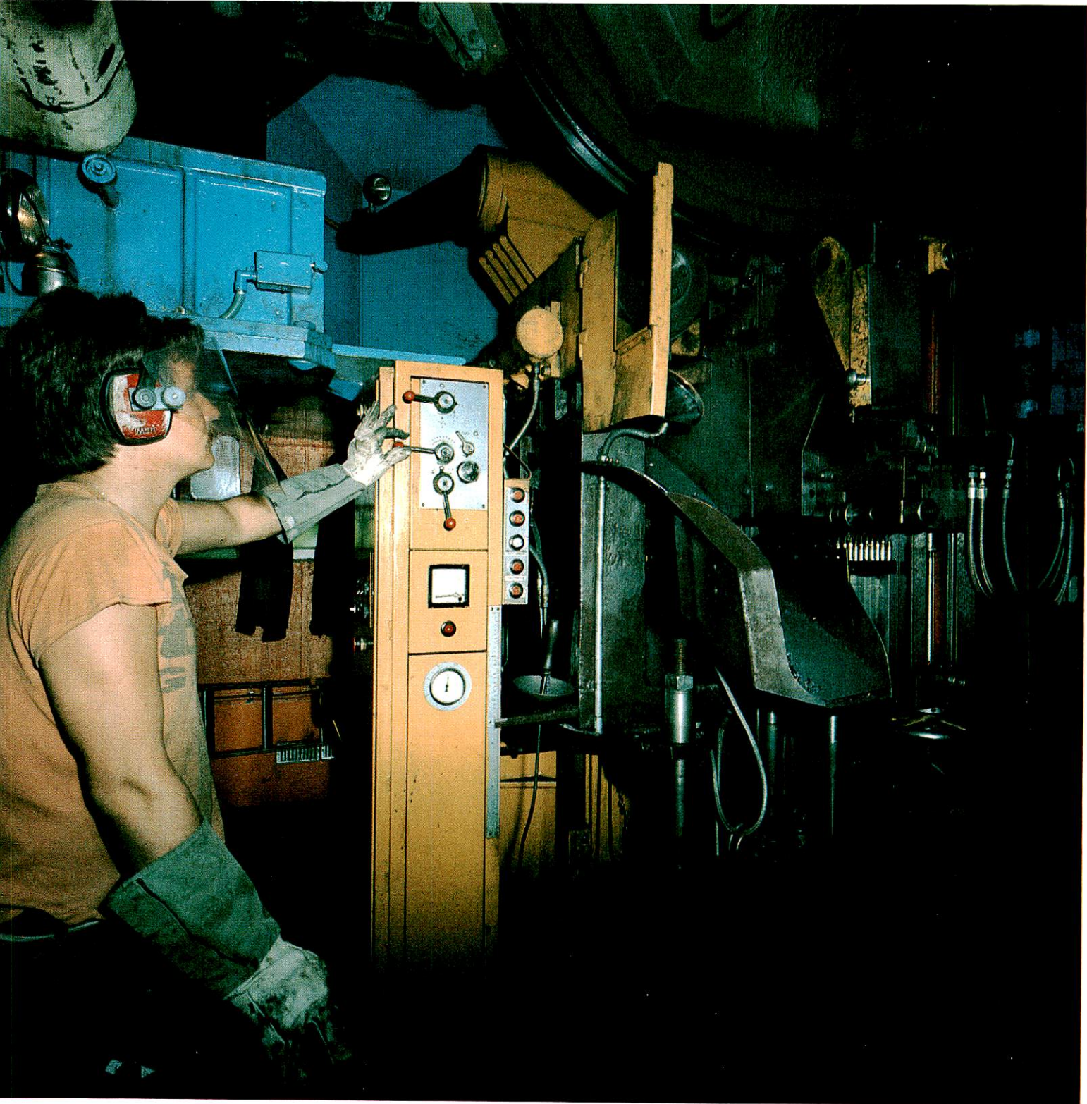
Locomotive wheels are turned on under-floor lathes, thus eliminating time-consuming wheel dismounting
