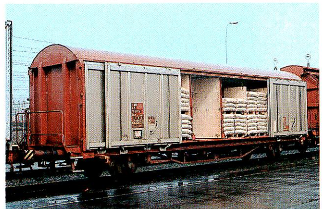
Class Hbis wagon with sliding side walls. Movable transverse partitions ensure steadier loads and allow maximum utilization of wagon capacity.
