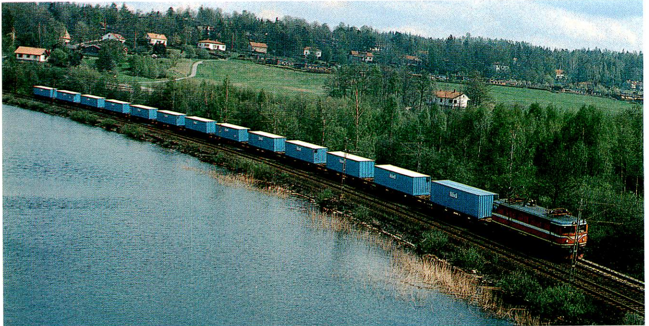
Long wagons accommodate six containers (two rows of three)
