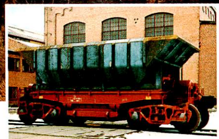
This ore wagon has a capacity of 80 tons. SJ also operates older 42-ton ore wagons.
